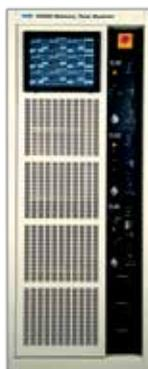
The NHR 9200 Battery Test System provides a battery mode allowing programming the series resistance ( $R_s$ ) and a no-load open circuit voltage ( $V_{ocv}$ ). When programmed, the system automatically adjusts the output terminal voltage based on the direction and level of current flowing to, or from, the charger.
