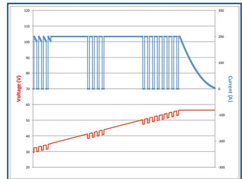
The voltage seen at the terminals of a battery decreases slightly as a charger reduces, or even reverses, the charge current. Similarly, the voltage at the terminals of a battery increases slightly as the charger supplies additional current. Both of these effects are caused by the internal resistance of the battery chemistry and the wire connections.
