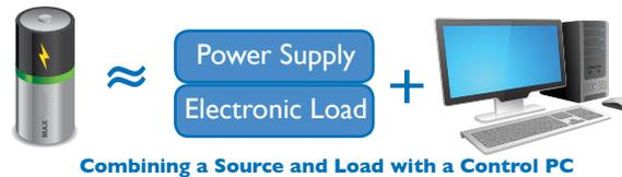
The PC can be programmed to control the power supply and load to emulate how a battery actually behaves any time the charger performs a “test” of the battery. In this case, the PC continuously measures the voltage and current being delivered by the charger then, as needed, adjust the power supply and load to emulate the battery’s response. This process is then repeated throughout the entire simulated charge profile.
